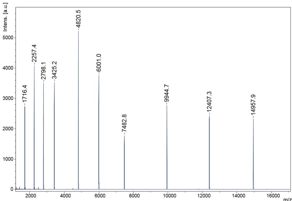
**Exhibit 2: SpheriCal® 10-point spectrum with CHCA matrix**
